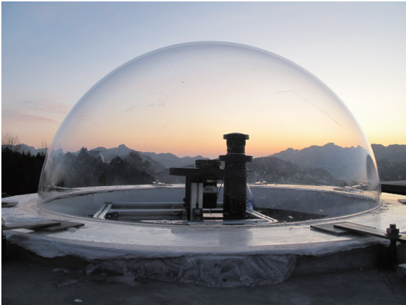
Figure 8. The all-sky imager installed by Prof. XU Jiyao and his colleagues from NSSC in Xinglong County, Hebei Province near Beijing.
