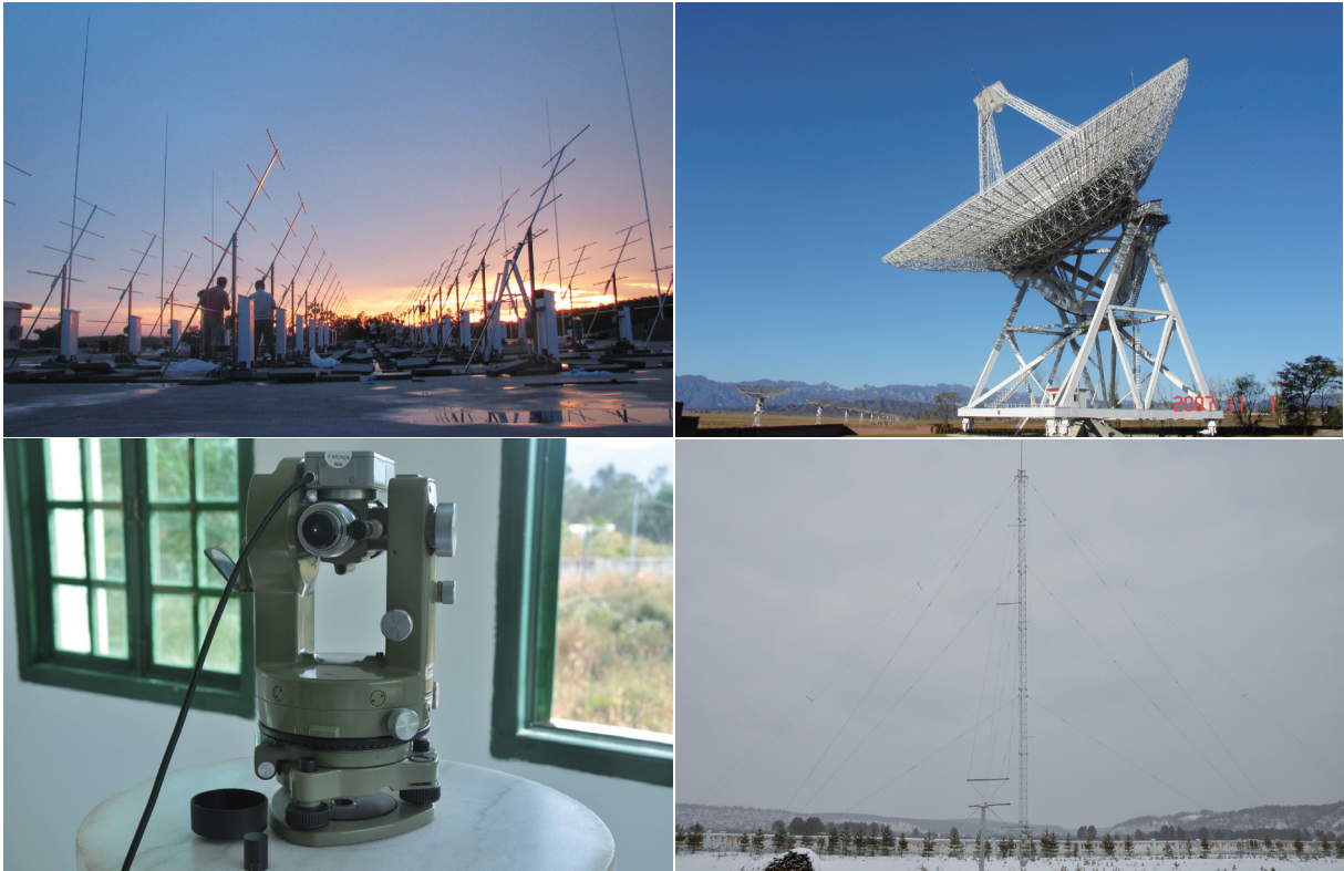
Figure 7. Some other instruments applied by the Meridian Project: (top left) the very high frequency radar array built by NSCC in Hainan, mainly for the monitoring of ionospheric variations; (top right) a radar facility built by the National Astronomical Observatories in Miyun County, suburban Beijing to detect interplanetary scintillations and measure the velocity of solar winds; (bottom left) a magnetic fluxgate theodolite; (bottom right) the digital ionosonde ( digisonde ) installed in northernmost China's Mohe City by the Institute of Geology and Geophysics, Chinese Academy of Science.
